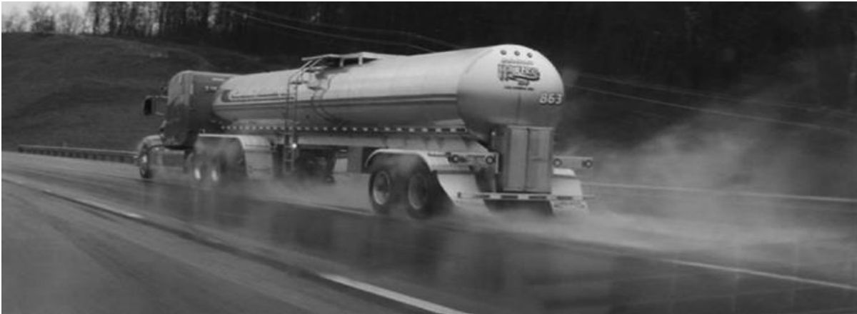
Figure 2 Issues Due to Inadequate Drainage in Pavement
